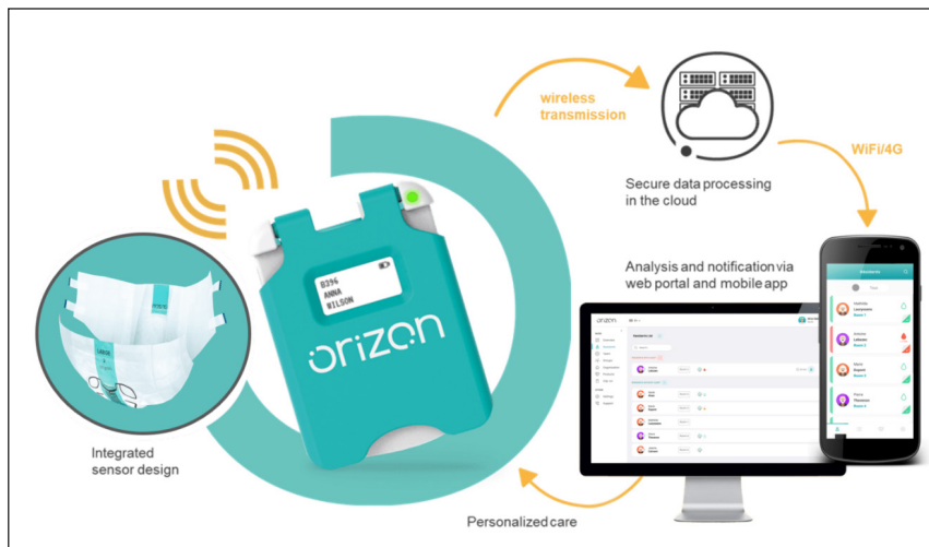
Figure 2. Data collected by the SMART sensor are transmitted via wifi to the cloud, making the information available for nurses to view on a smartphone or desktop computer
